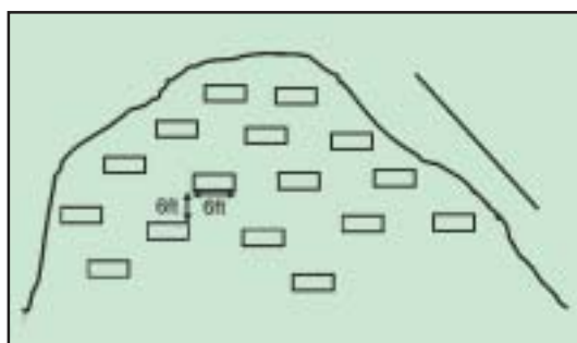
Figure 5.2 Staggered trenches along a slope.
